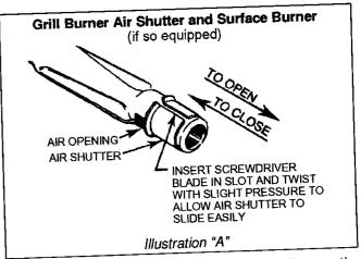
On any burner, closing the air shutter too far will cause the flame to become soft and yellow tipped. Opening the air shutter too wide will cause the flame to blow away from the burner ports. Proper adjustment will produce a sharp, clearly defined, even blue flame.
